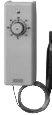
The TY6800Z and TTY6800Z are thermostats with a remote sensor that can be inserted into an air duct or into liquid in a tank or pipe. These devices automatically control solenoid valves, motor valves, electric heaters, compressor motors for air conditioning equipment or heating/cooling equipment, etc.
